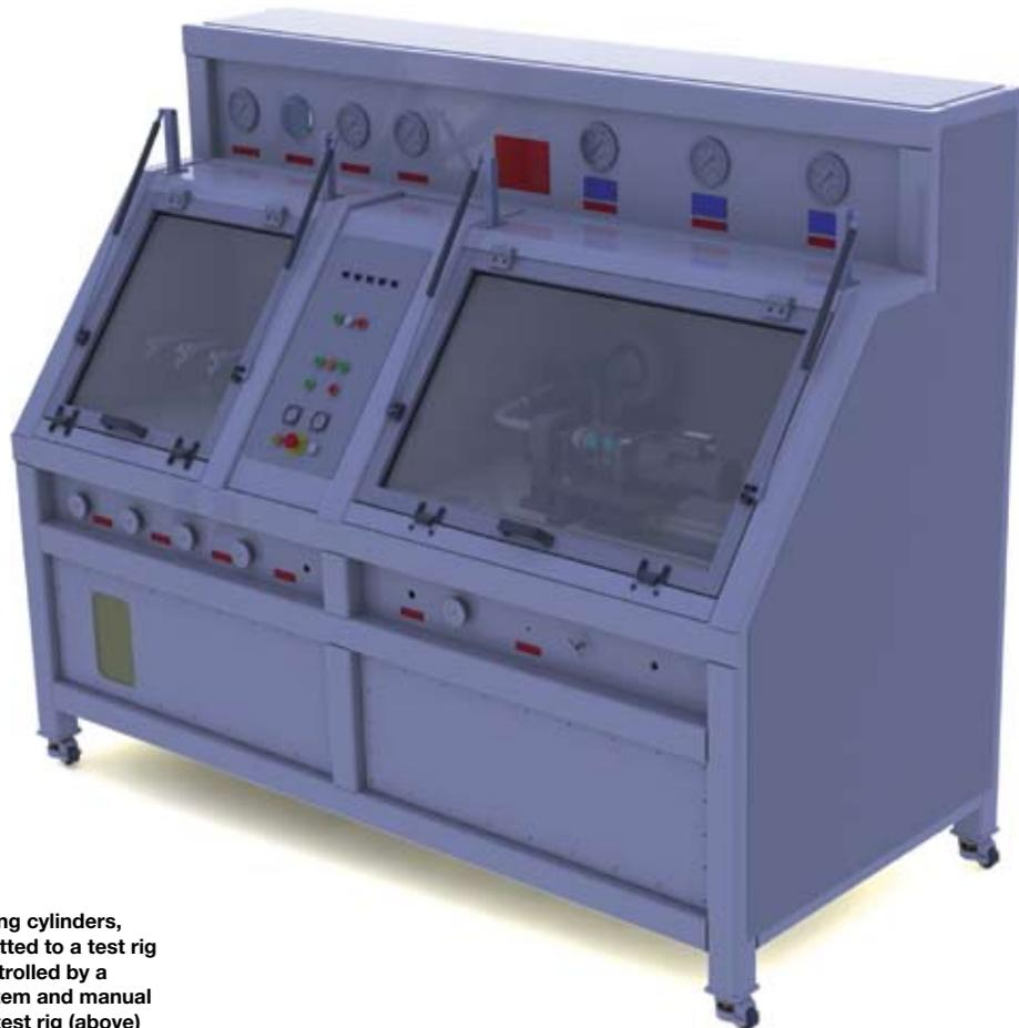
Servo loading cylinders, which are fitted to a test rig but are controlled by a central system and manual hand wind test rig (above)
